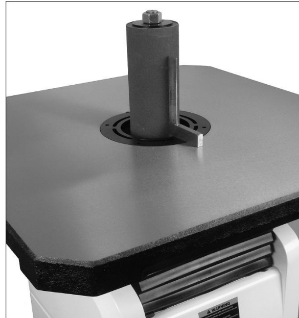
Figure 13: setting tilt stop
